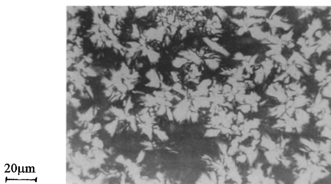
Figure 8. Photomicrograph of the (25/75)/40 (iPP/HDPE)/HOCP blend, isothermally crystallized for 900 min. at 125°C (polarized light).
