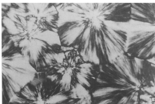
Figure 4. Photomicrograph of the 100/0 iPP/HDPE blend, isothermally crystallized for 3 min. at 125°C (polarized light).
